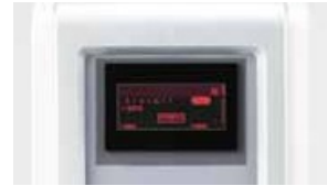
Green screen during operation, red screen when alarm occurs
