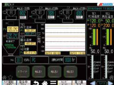
Trend graph Operation history of the dryer can be seen at a glance.
